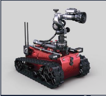
WATER / FOAM MONITOR
