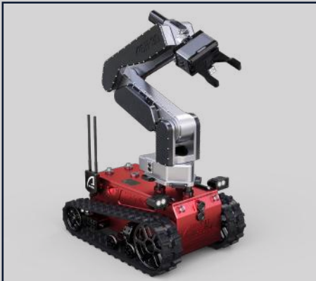
ARM (LIFT CAPACITY: 70 KG / 154 LBS)
